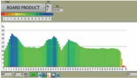
View graphic profiles in multi-deck displays, cross-direction moisture profiles, bar graphs, and more.
