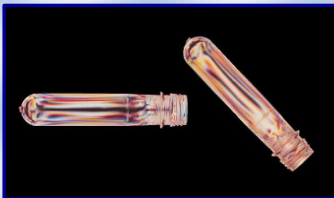
Parallel view and 45° view of preform by PL-P
