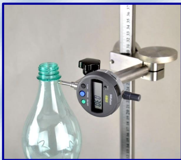
Ruler allows accurate measuring
