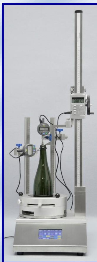
UBPT-3 with 3 measuring heads (for mouth clearance, perpendicularity & height) and integrated double automatic calculators
