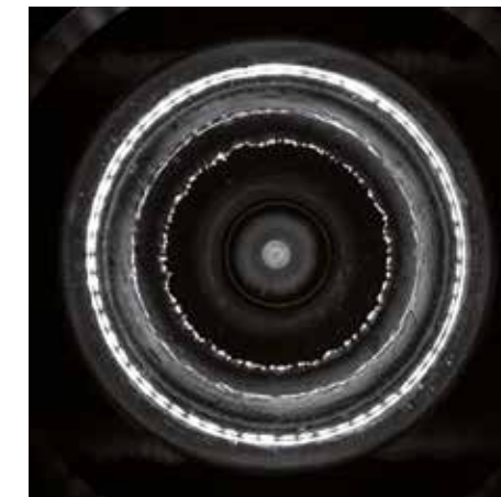
PET bottle: stress cracks, resulting in leakage
