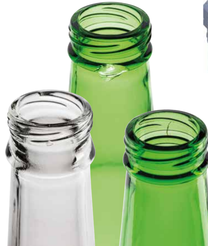
Twist-Crown: Thread defect
