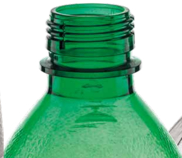
Abrasion through faulty neck ring guide
