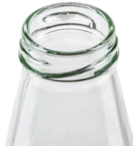
Twist-Off: Thread defect
