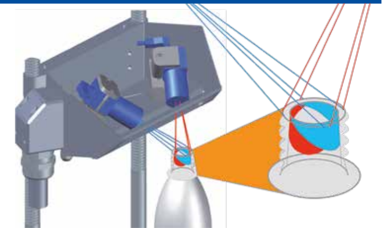
miho FSI schematic view: the cameras look down at an angle from above into the finish
