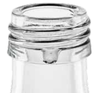
MCA: Chipping at the flanged edge
