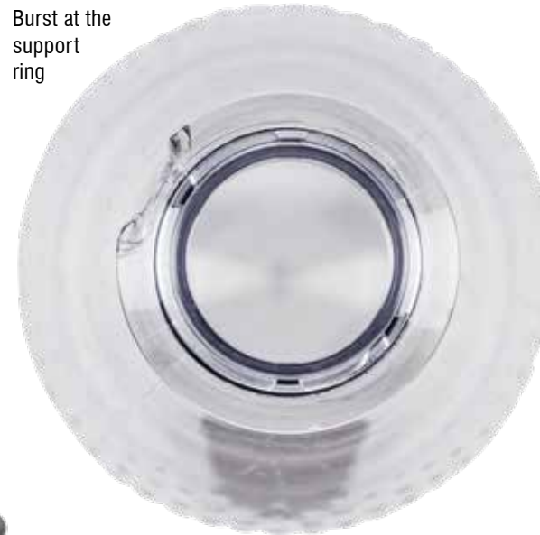
PET bottle: stress cracks, resulting in leakage
