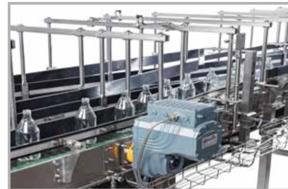
Two-sided rail adjustment
